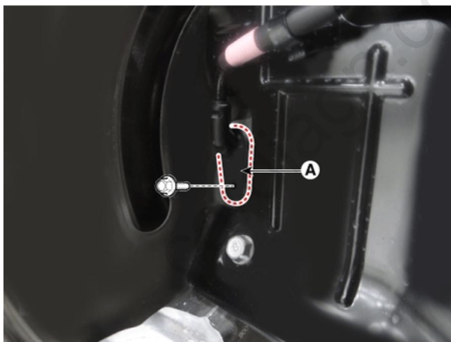
14. Remove the brake cooling cover (A).
