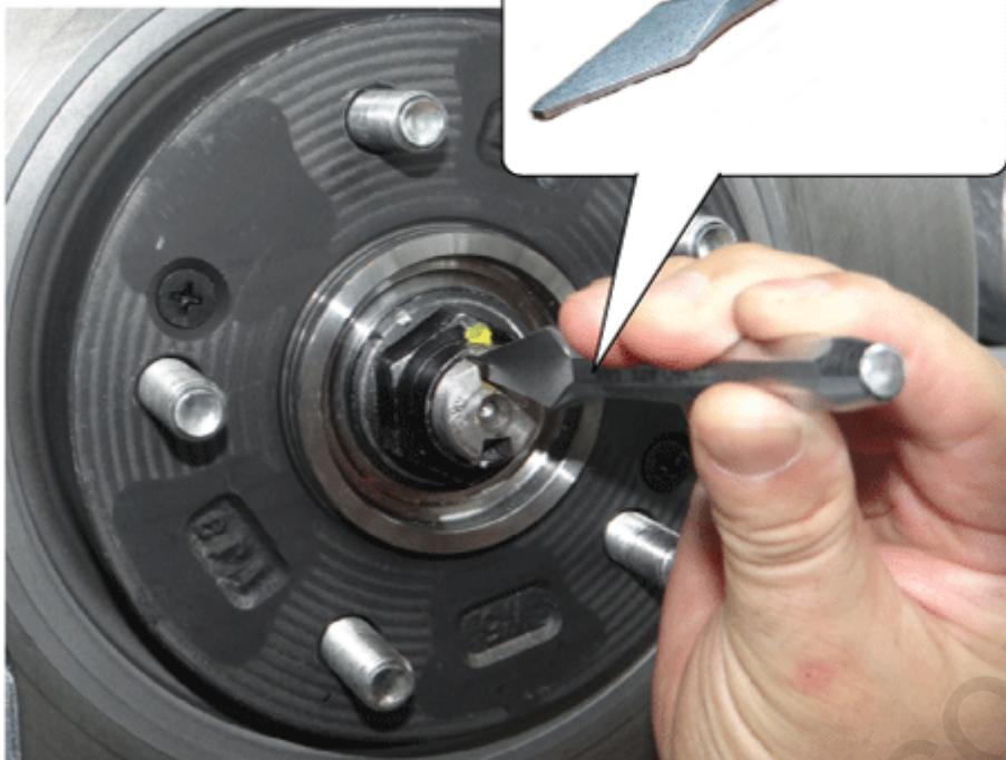
12. Loosen the caulking nut (A) and then separate the hub assembly from the drive shaft.
