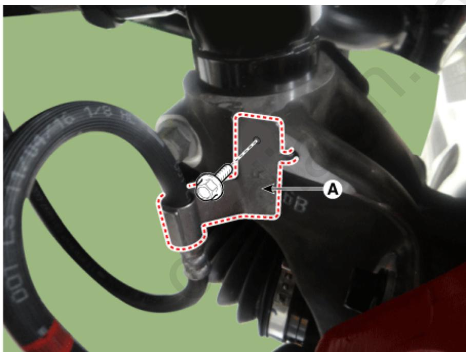
11. By hammering on a chisel, unlock the driveshaft lock hub nut caulking.
