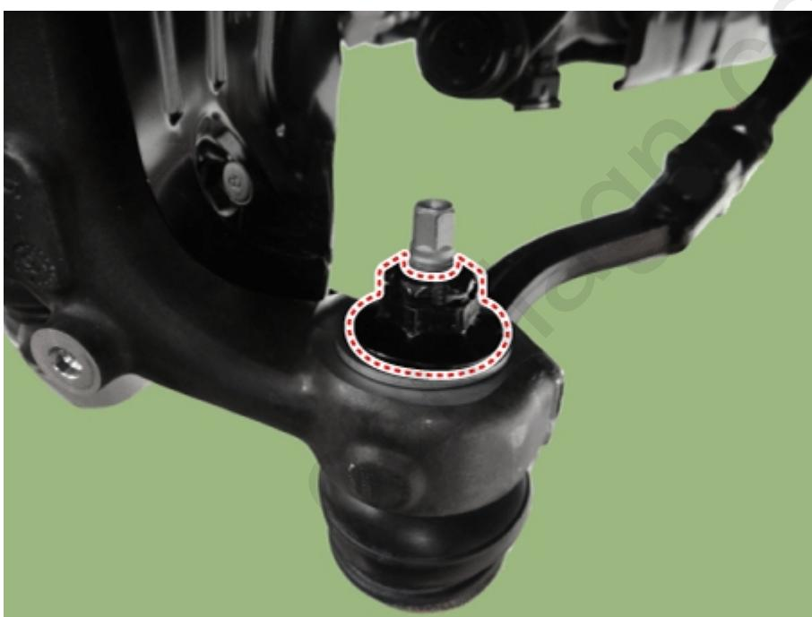
9. Remove the knuckle by using the ball joint remover (A).
