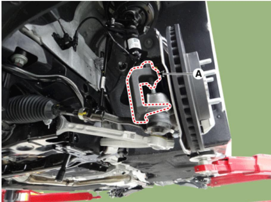
10. Remove the brake hose bracket (A).
