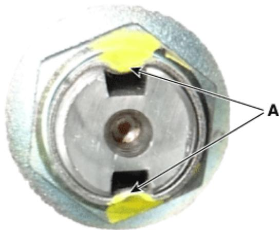
13. Loosen the wheel speed sensor bolt (A) and then disconnect the wheel speed sensor.
